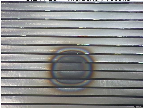
Upstream side after \sim 3.2 \times 10^{21} Incident Protons
