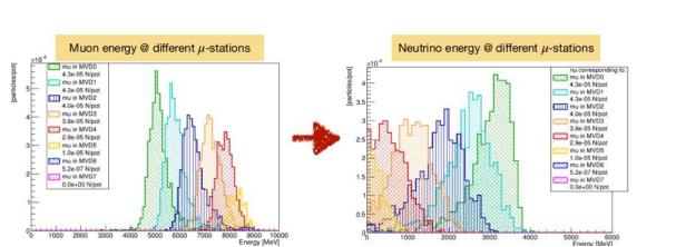
Hottest detector (upstream station): cope with ~2 MHz/cm<sup>2</sup> muon rate and ~10<sup>12</sup> 1 MeV-n<sub>eq</sub>/cm<sup>2</sup>
