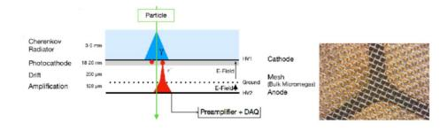
Possible candidates: fast Micromega detectors with Cherenkov radiators (PIMENT)
