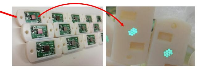
SiPMs installed outside of calorimeter, above shielding: avoid hadronic shower and reduce (factor 18) aging
