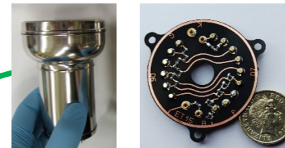
1/3 TPC PMTs Xenon PMT bases
