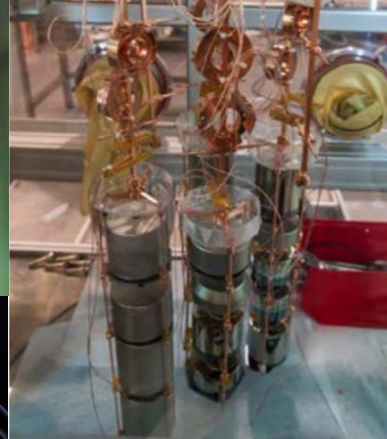
LEGEND-200 integration tests 20 detectors / 4 strings
