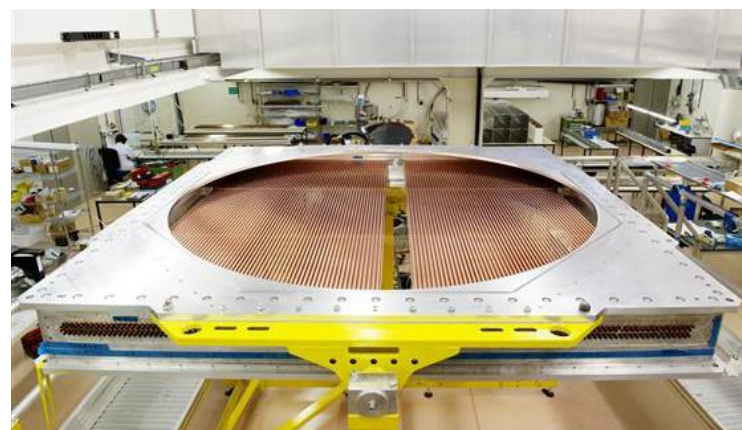
A current NA62 STRAW chamber
