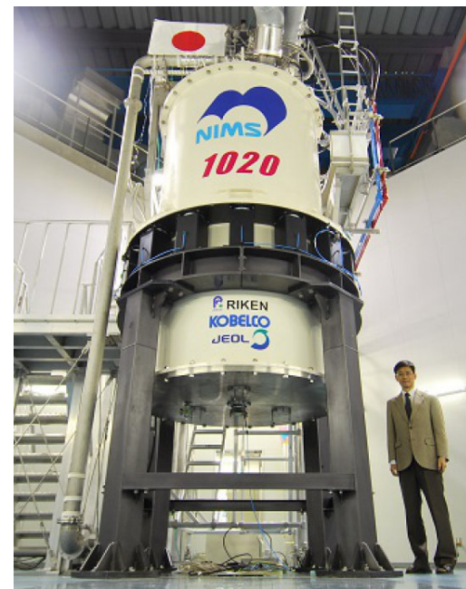
1020 MHz NMR using 24T at 2.2K
