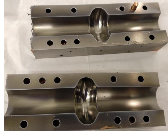
6 GHz split cavity with Nb coating
