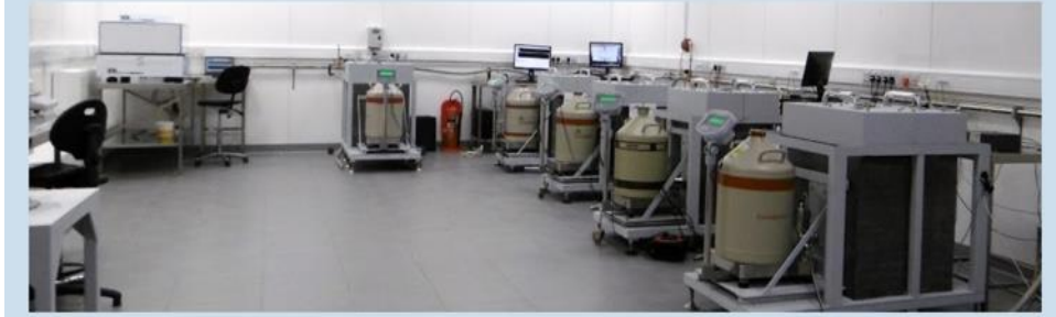
BUGS (UG): A range of HPGe detectors and alpha particle detectors for intrinsic and surface radioactivity measurements.
