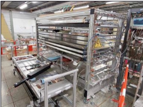
Setup for cosmics with new muon chambers
