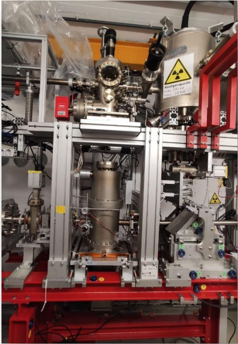
Small Thermalized Electron Source at Mainz
