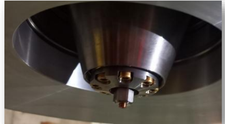
Target nozzle with 20 \mu\text{m} diameter
