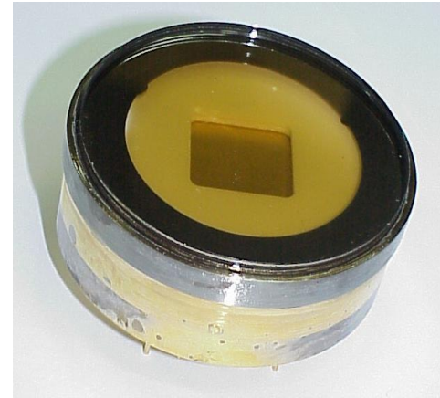
GEM with semi-transparent Photocathode (K-Cs-Sb)
