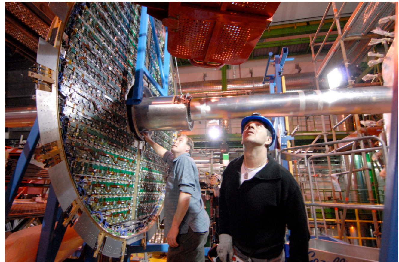
Preshower Dees positioned around beam pipe
