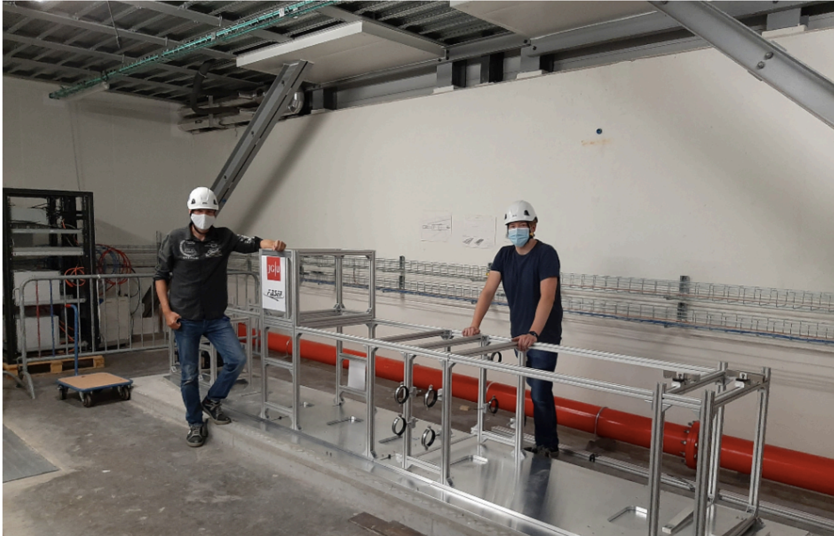
Assembly test of the upper frame on the upper and lower baseplate in the FASER test lab in Preveessin
