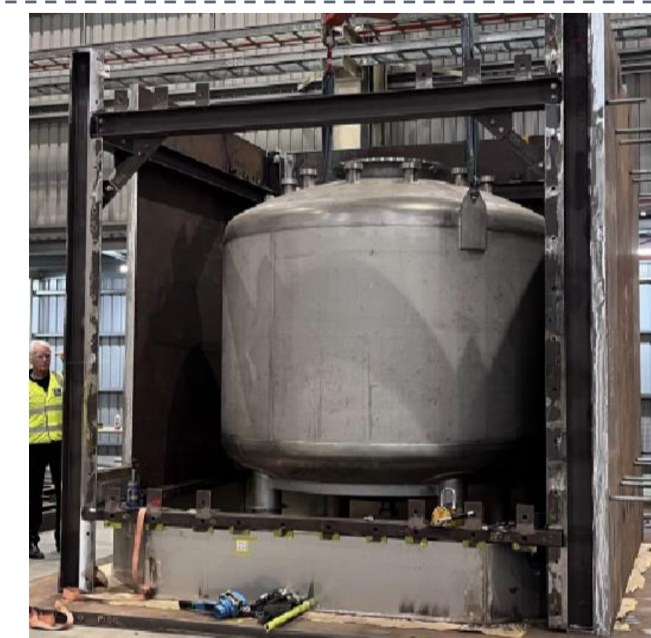
Figure 2.2: Test assembly of the shielding and veto vessel completed above ground.
