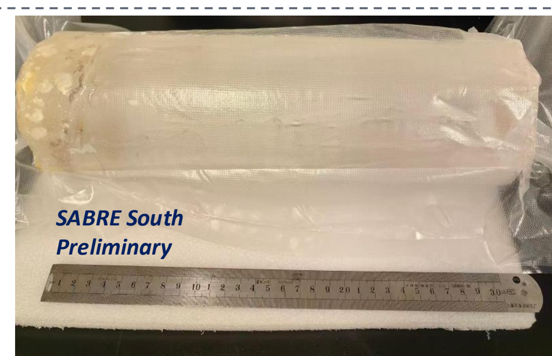
Figure 4.2: First successfully grown production-level NaI(Tl) crystal, grown from 10 kg of powder, weighing approximately 7 kg
