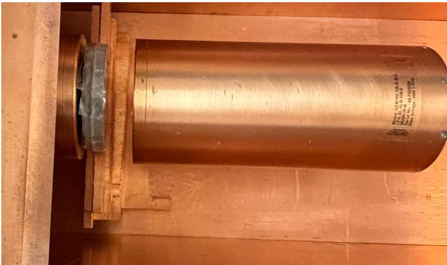
Figure 4: Picture of the opened Twins system with a petri dish of TML between the crystals, with the SL on the right, and the HJ on the left.
