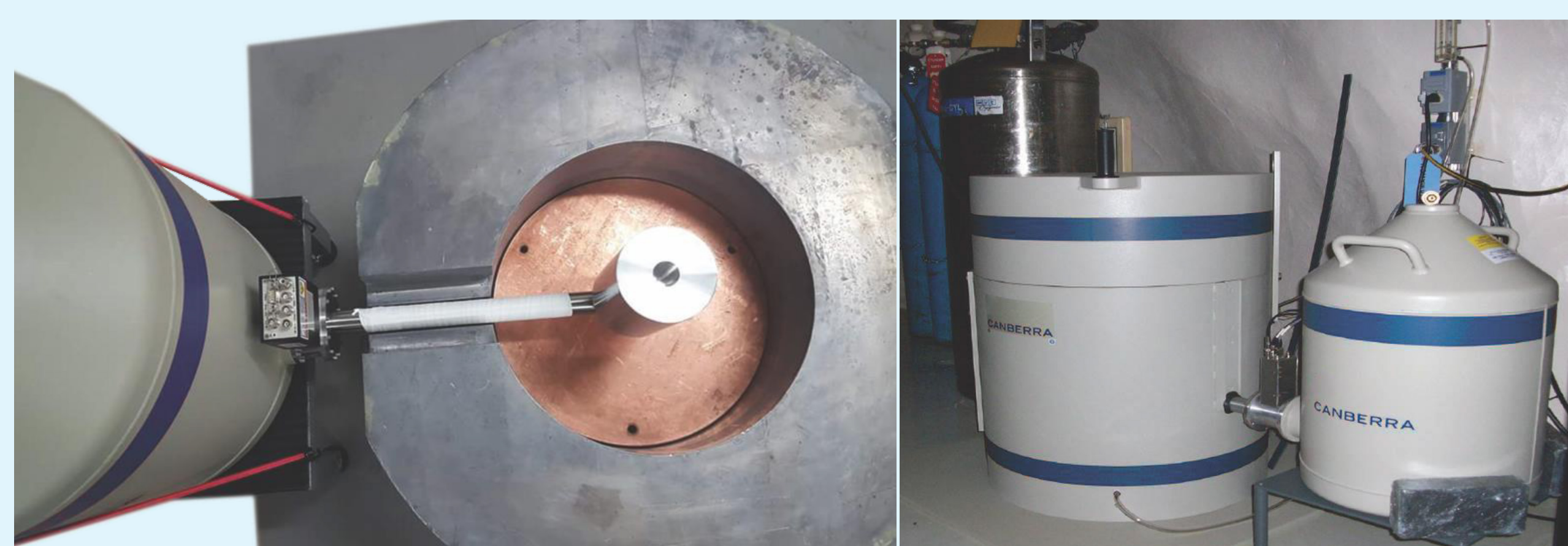
SAGe Well detector installed inside a lead castle
