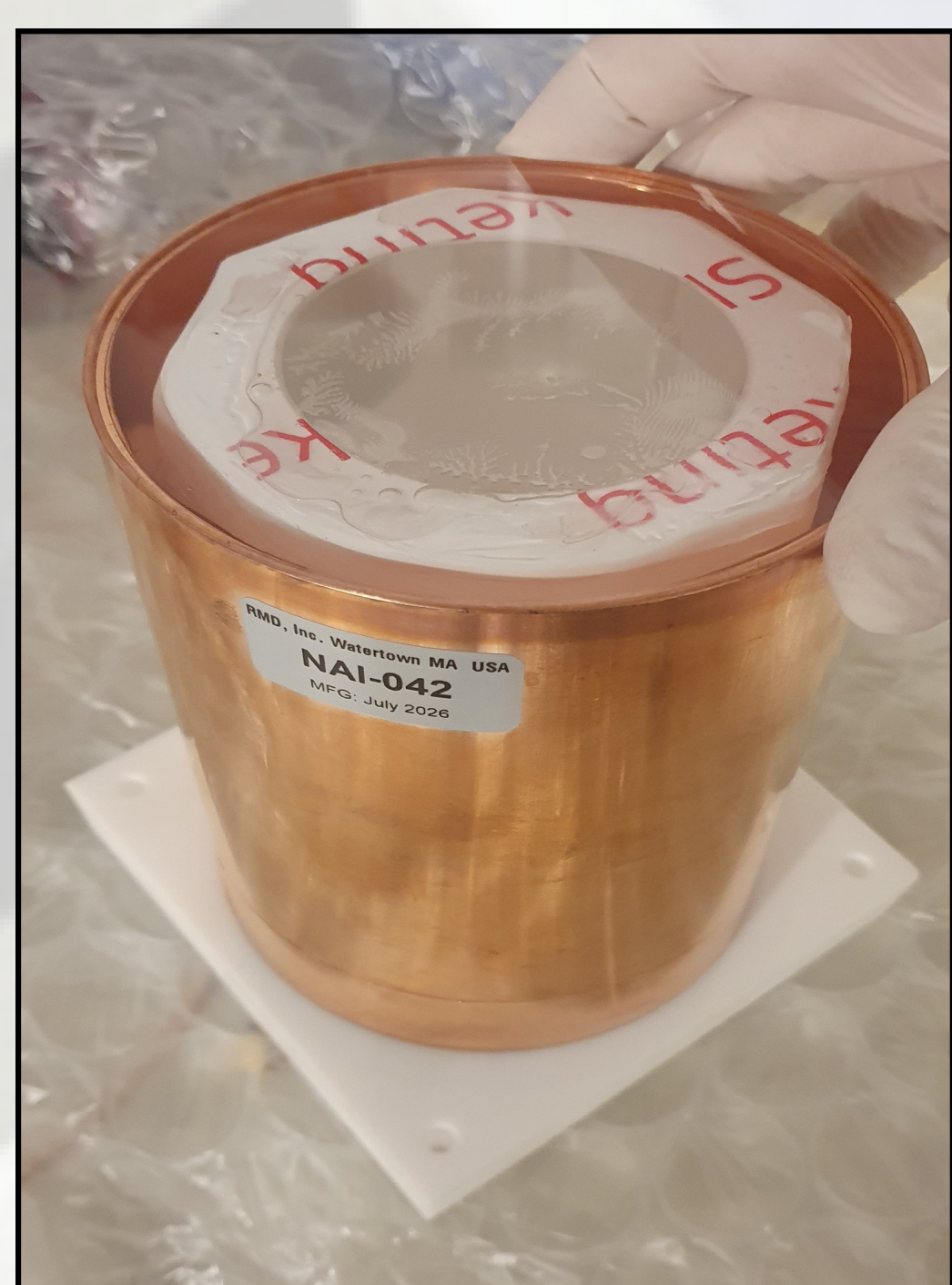
Crystal NaI-42 encapsulated in copper.
