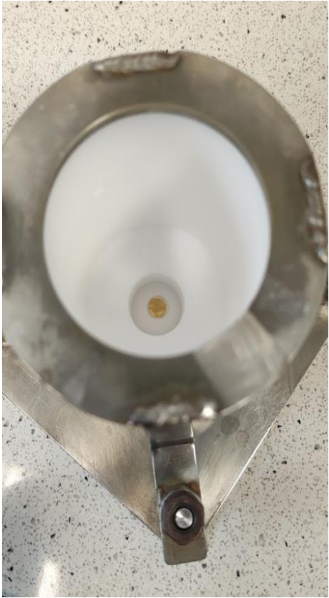
PTFE electroplating cell used for Po deposition
