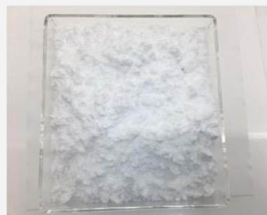
3. synthesis of ammonium polymolybdate powder and its annealing 4. final ^{100}\text{MoO}_3 powder
