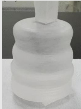
2.5 inch test Kyropoulos growth (CUP, Korea)
