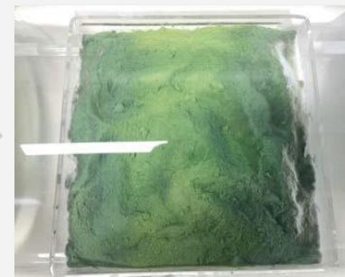
3. synthesis of ammonium polymolybdate powder and its annealing 4. final ^{100}\text{MoO}_3 powder
