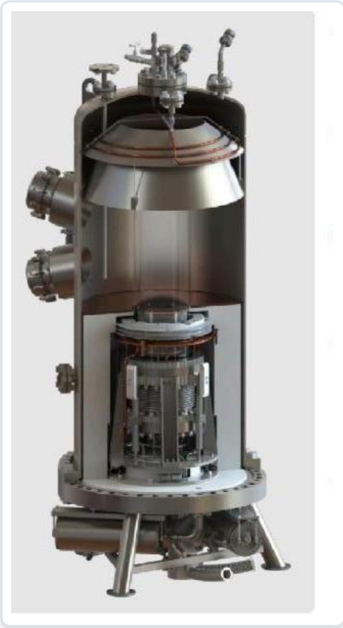
PICO-40L in the right-side-up (RSU) configuration.
