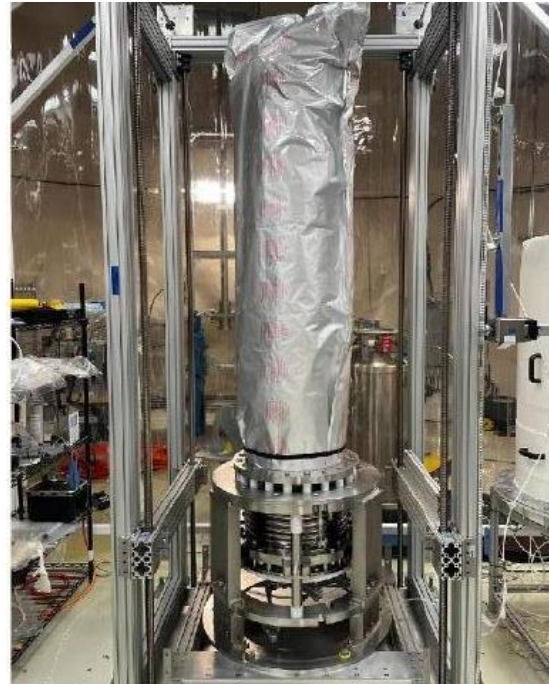
The silica jar, wrapped for low-background installation.
