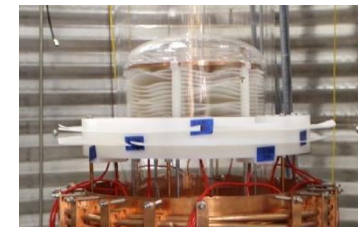
Piezo transducers (left) mounted on the PICO-40L instrumentation ring (right)
