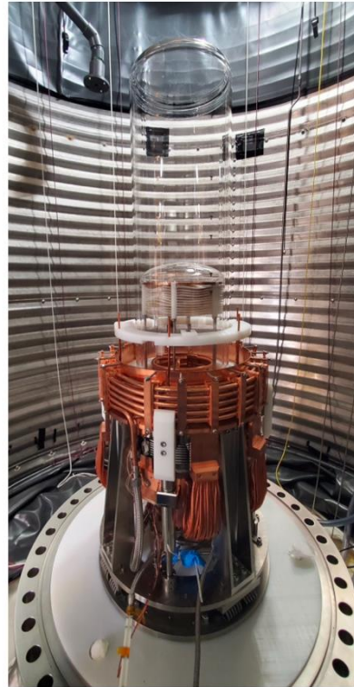
The assembled inner detector as installed underground at SNOLAB.
