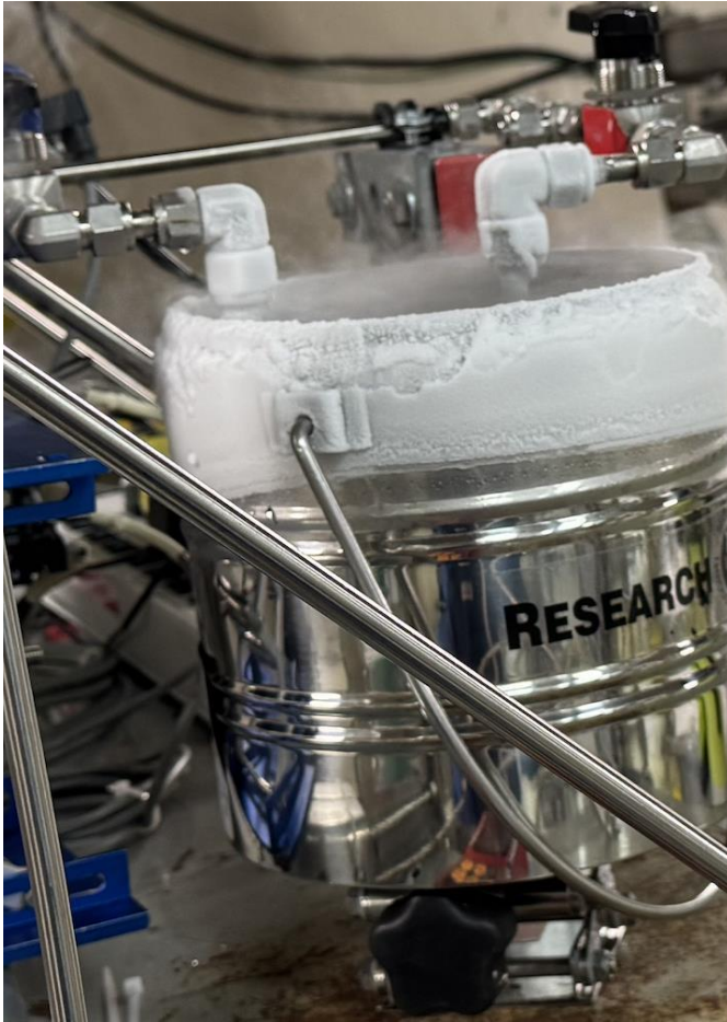
The hybrid trap's charcoal stage submerged in \text{LN}_2 during cryo-adsorption.
