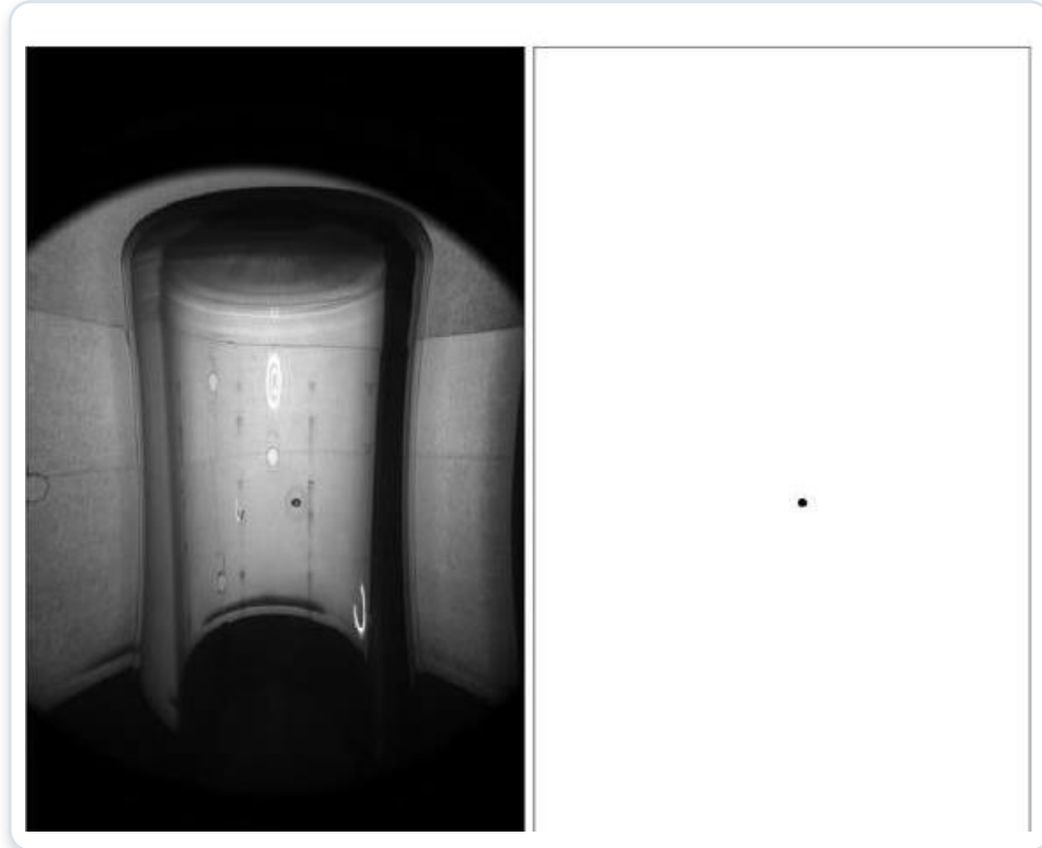
Raw fisheye frame: a bubble appears as a bright glint. After Processing, reduced to a single (x, y) position.
