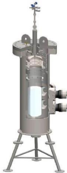
PICO-60 35 L of CF_3I and C_3F_8 2016–2017
