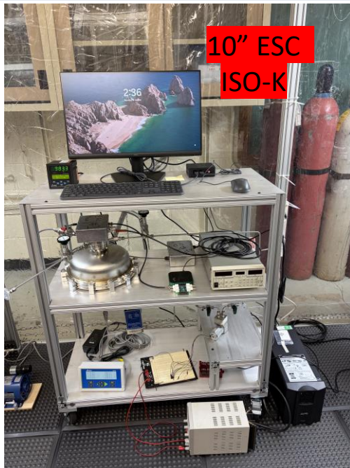
Recirculating ESC gas system
