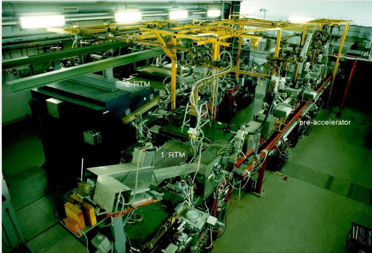
RTM1 and RTM2 for 180 MeV beam energy
