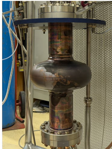
KEK14, KEK15 Brazed and welded with CF flanges
