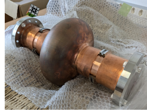
C1c, C1d Hydroforming + Plasma EP
