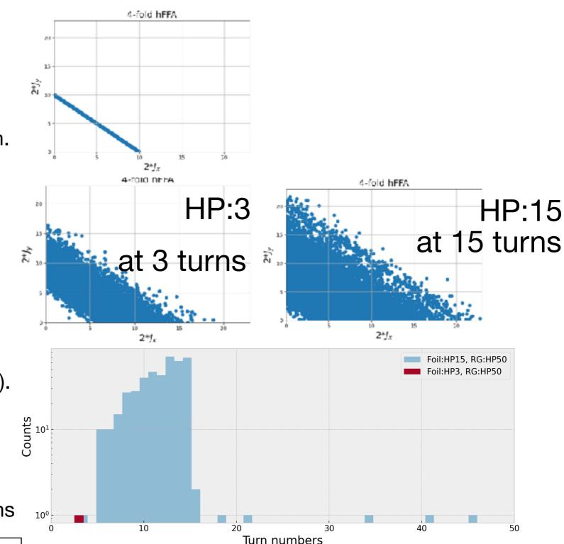
Turn numbers the particle reached  $250\pi mm.mrad$  over 50turns when the beams hit the foil for first 3 and 15 turns, corresponding to the hitting probability of 3 and 15 respectively.
