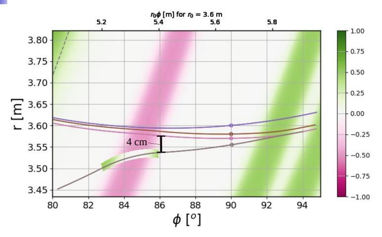
4 cm between edge of proton beam and H- injected beam
