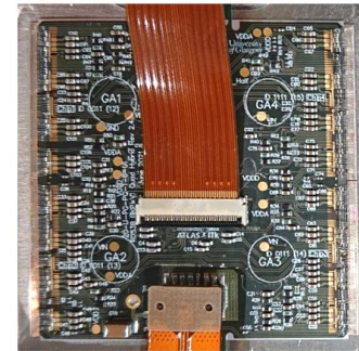
Quad module: 1 quad-size sensor tile ( \sim 4 \times 4 \text{ cm}^2 ) and 4 frontend (FE) chips
