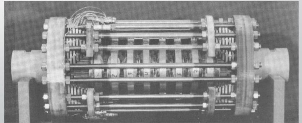
D1 magnet prototype produced by Karlsruhe Laboratory (1973)
