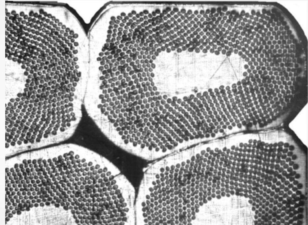
Compaction to align with the magnet design
