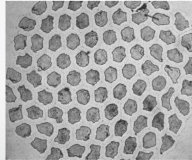
**100 Micrometer NbTi filaments embedded within a copper Matrix.**
