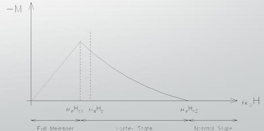
Figure 2.4: Magnetization curve for a type-II superconductor.
