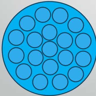
Self-field effects are limited to the inner and outermost filaments when twisted
