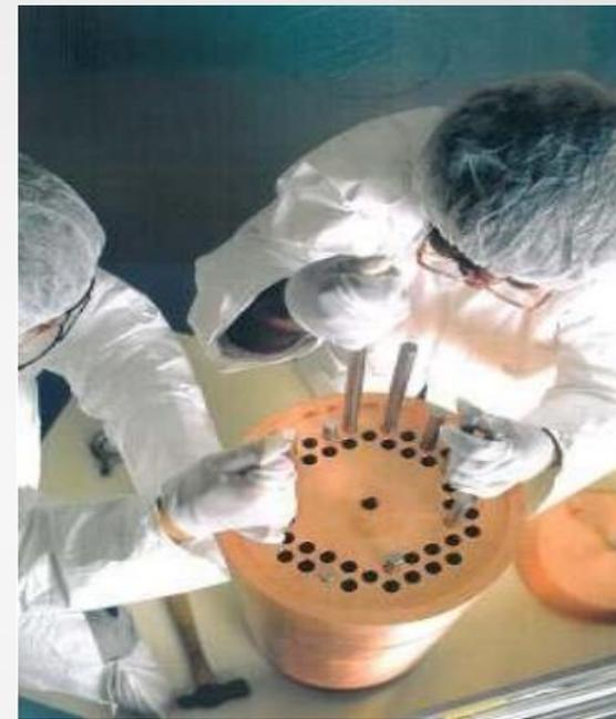
NbTi rod insertion into copper billet at Intermagnetics General Corp. Image credit: IGC
