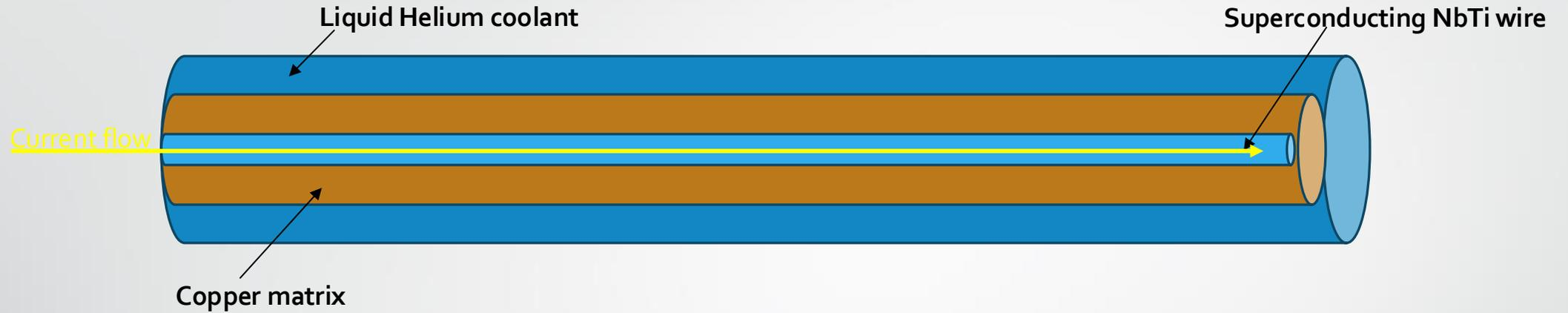
Normal state: Liquid Helium coolant surrounds the copper conductor; the superconducting filament is kept below its critical temperature.
