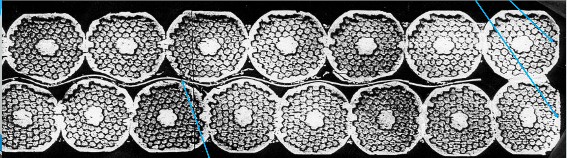
Oxide layer between wires
