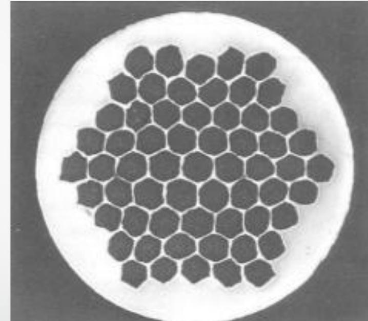
Prototype coil manufactured in 1967 by the IMI and RAL collaboration. This singular strand consisted of 61 50µm filaments (black polygons) within a conductive matrix (white surroundings).
