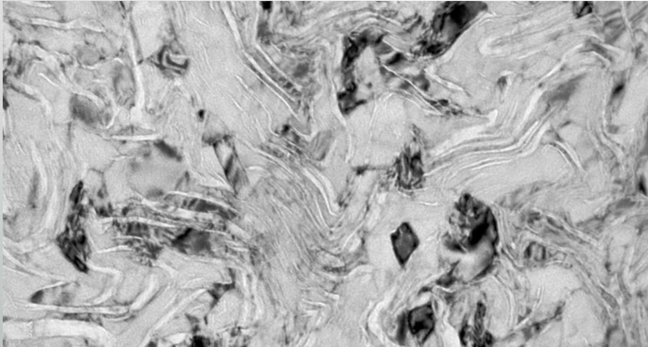
**NbTi alloy:** Transmission electron microscope image of a NbTi filament.
