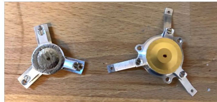
Left: ^{100}\text{Mo} target, Right: ^{197}\text{Au} stopper – after conclusion of beamtime.
