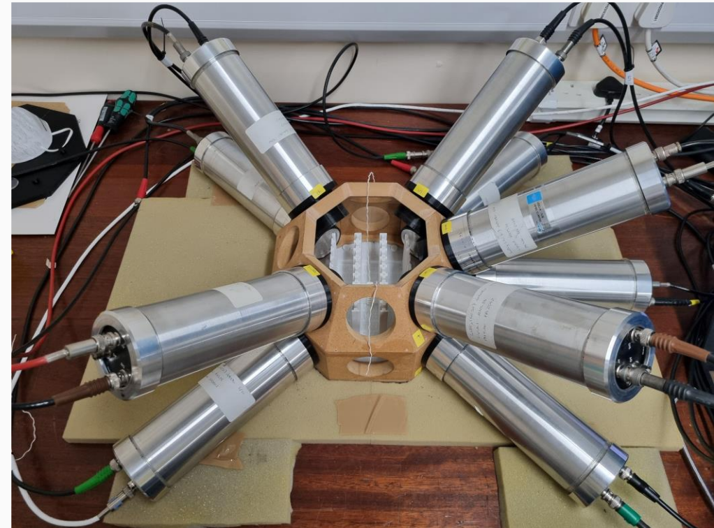
Fig 13. Photograph of the experimental setup of the 10 detector array.
