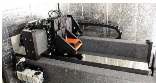
Fig. 1: left: a view inside the metrology box of the BESSY large volume AFM, right: AFM-measurement result taken at a highly contaminated synchrotron mirror
