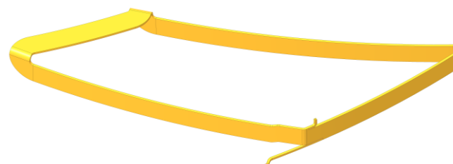
Single trim coil wound with □10mm conductor with Ø6mm hole
