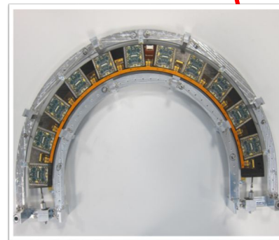
RAL is one of 4 sites loading pixel modules onto 3 sizes of half-ring structures
