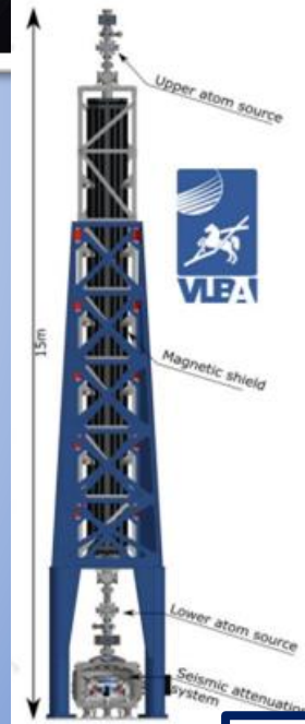
VLBAI: Terrestrial tower using atom interferometer O(10m) (Germany)
