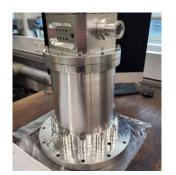
AGATA – design and production of a source holder for the self-calibration technique measurement.
