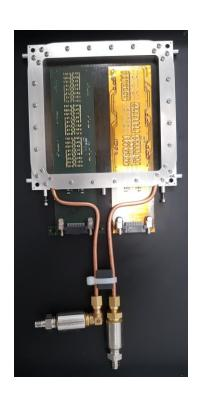
New motorised target system and motorised beam blocker assembled at CERN after an assembly test at DL.
