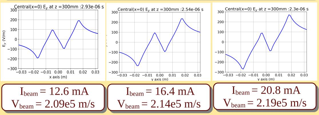
The vertical electric field profiles at 300 mm, mimicking the U<sub>ext</sub>(Extraction conditions of Voltage) rise (6, 7, 8 kV), calculated Child's using the Langmuir law, and scaled down.
