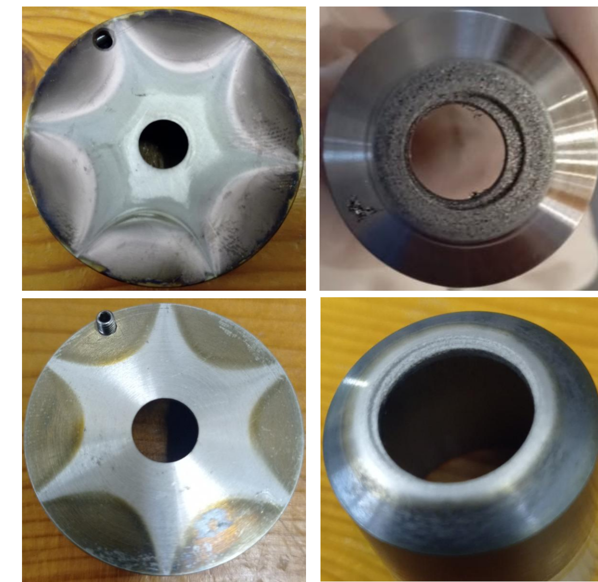
Figure 5: Increase in plasma electrode (left) diameter from 6 to 8 mm, and extraction electrode (right) diameter from 8 to 12 mm
