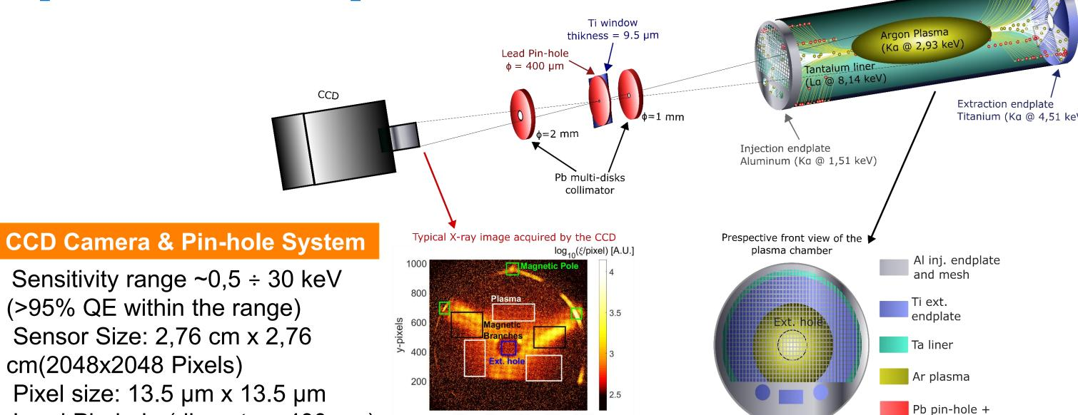
Lead Pin-hole (diameters 400 µm) Lead multi-disks collimator system
