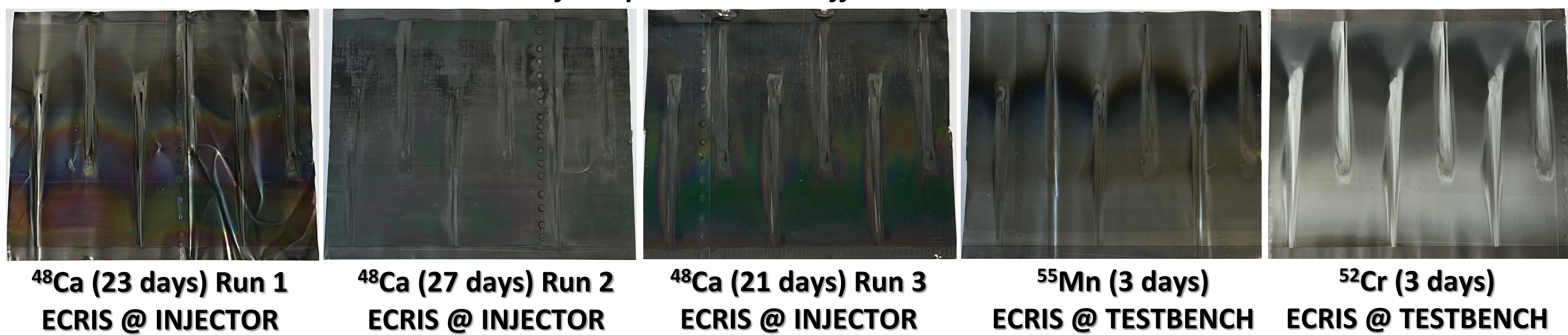
Ta liners after operation with different metallic elements
