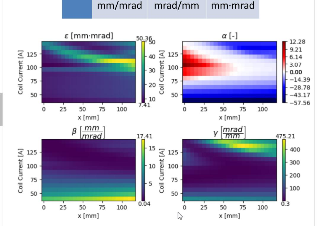
Achieving the needed beam emittance and Twiss parameter values is possible, but the solenoids must be positioned **directly** before the RFQ.
