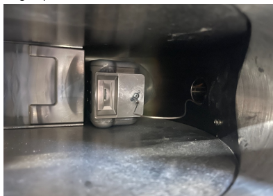
Fig. 2: An inside view of the vacuum box and extraction slit from the ion source.
