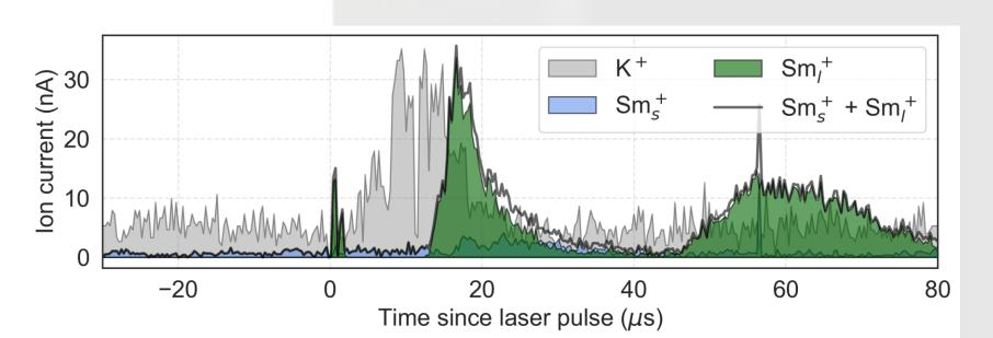
A simulated time-structure profile with a 40 ns laser pulse at time stamp 0 µs.
