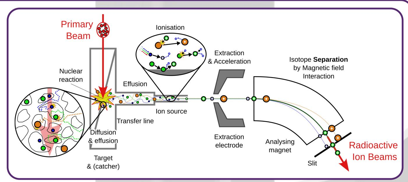
ISOL technique diagram which combines target bombardment, release, ionization, extraction and acceleration [4].
