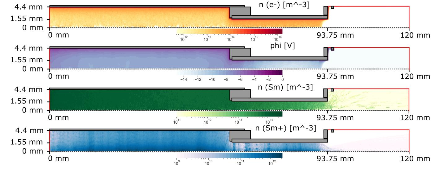
Simulated  $n_{e-}$ ,  $n_{Sm+}$  and  $\phi$  profiles in a hot cavity ion source.
