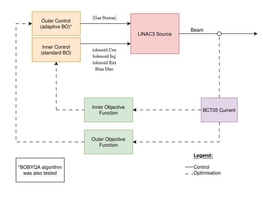
Hierarchical controller: only 2 fast actors and gas injection acquisition shown for clarity.
