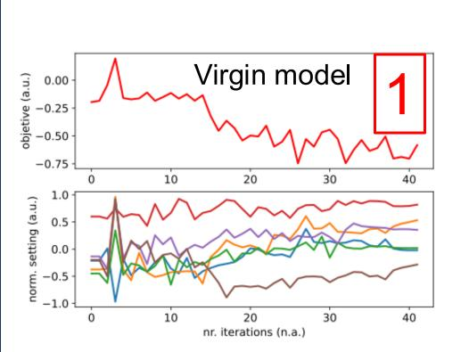
Results of successful recovery test from detuned source. BO with different exploration settings  $(\beta)$ .
