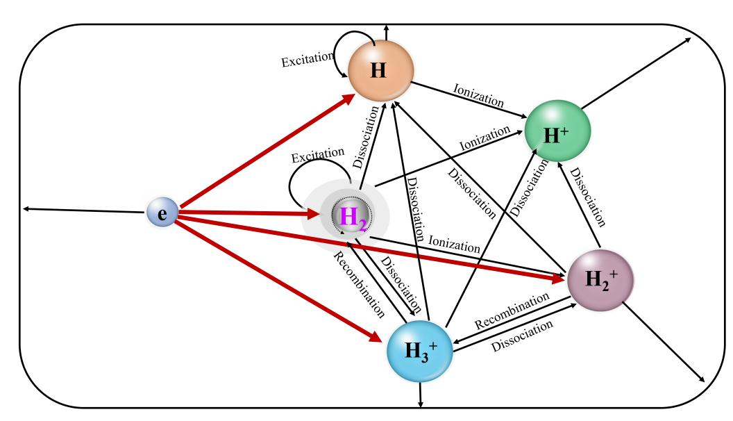
Fig. 1 Schematic diagram of main reaction processes in hydrogen plasma
