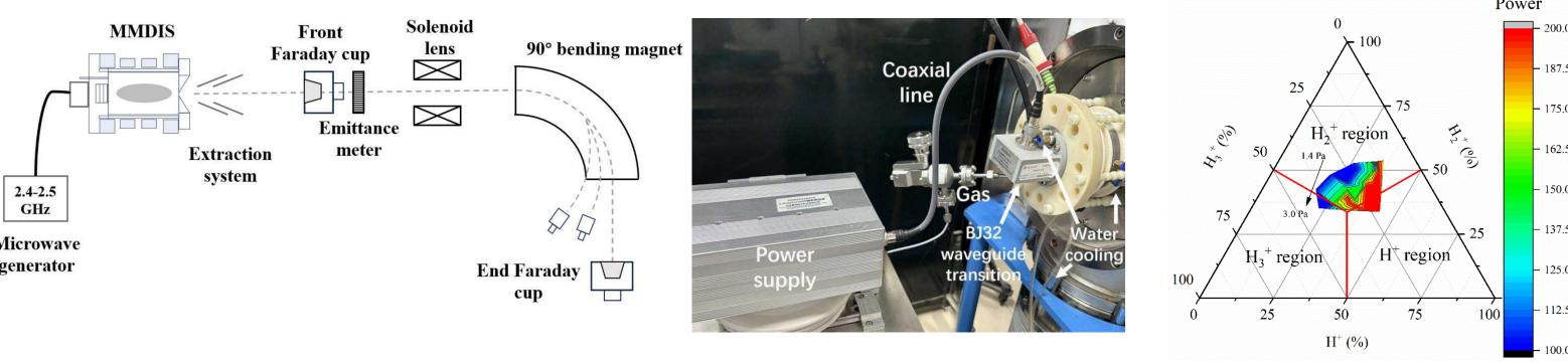
Fig 8. Schematic of experimental system
