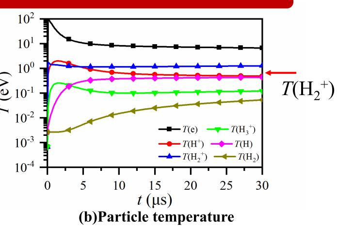
Fig 2. Transition variation diagram of particle number density and particle temperature
