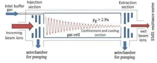
Ions drift to extraction thanks to a small electrostatic field; four RFQ rods are divided in 10 or 18 segments each. After RFQC, ions are reaccelerated with electrostatic fields towards the emittance meter.
