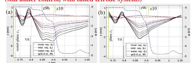
Restarted rays for (a) second and (b) first tetrode design, with  $V_9$ =-300 V and  $V_{9b}$ =-1.4 kV, and  $\mu_x$ =2 . Other resampling methods in development
