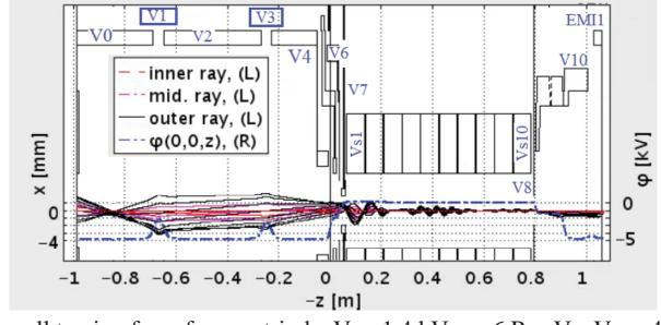
Overall tracing for reference triode  $V_9$ =-1.4 kV,  $p_g$ =6 Pa,  $V_0$ = $V_{10}$ =-4.8 kV
