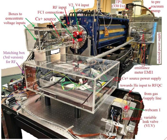
Overview of setup status, with Cs+ source and He leak valve VLV in the foreground (see also views on the right)
