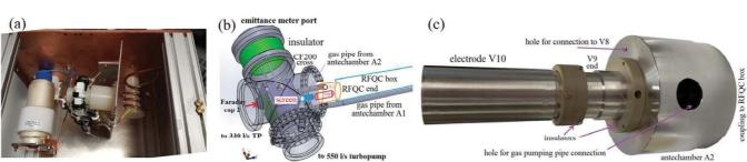
RFQC (from JPCS2022): (a) low power matching box; (b) scheme of emittance meter and pumps; (c) view of triode extraction line
