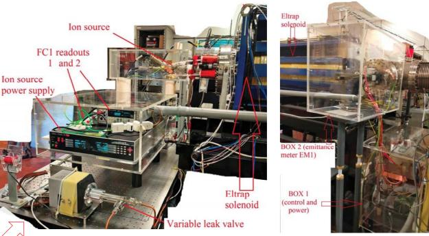
View of RFQC/Eltrap input setup, note leak valve, its tubes, and source turn on
