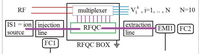
Block scheme of RFQC test parts (Eltrap setup); a multiplexer distributes RF and DC bias voltages to each RFQC electrode
