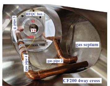
View of gas pipes and septum inside the 4way CF200 cross, with electrodes V9 and V10 dismounted from antechamber A2 to show V8.
