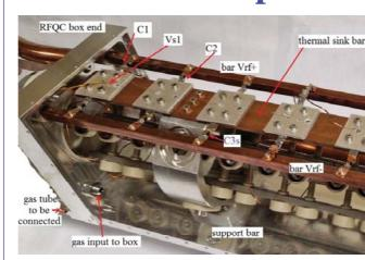
Detail of RF multiplexer (gas-tight RFQC cover removed); the resistors are sandwiched between mica foils for heat disposal towards a large copper bar; capacitors as C1, C2 and C3s stay in He gas region.
