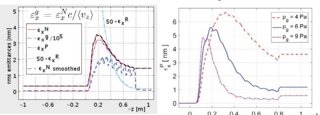
(a) Overall emittances in optimistic  $\mu_x$ =1 case, and initial  $\epsilon_x$ R=0.33 nm for  $p_g$ =6 Pa; (b) pencil emittances for several  $p_g$ Note that at extraction ray emittance is completely damped, but pencil emittance is not. It is thus convenient to restart rays with a multiplicative safety factor  $\mu_x$  > 2, to get a more realistic value of  $\epsilon_x$ N (still under control, with tuned tetrode systems)
