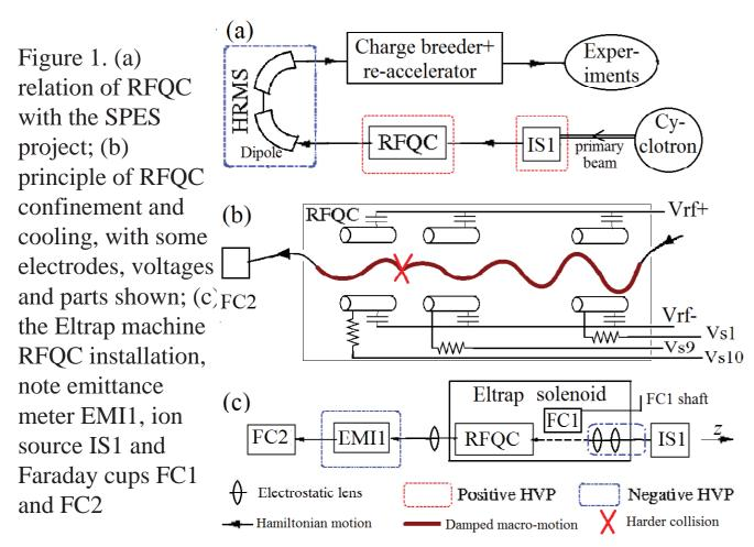
Cooler size and detailed shape depend from the spread amount to cool. For muon cooling spread is 100 MeV/c order so cooler length is 100 m order. In the case of exotic ions, produced by a fission target and the following plasma ion sources, the rms energy spread is in the 5 eVrms order, so cooler length is about 1 m.
