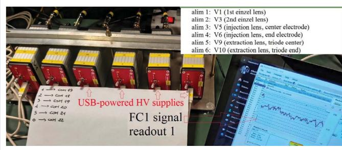
An array of some HV supplies for beam lenses (usually needing more voltages each, but for so-called einzel lenses); their regulation allows to changes slightly current in FC1 (wireless readout shown)
