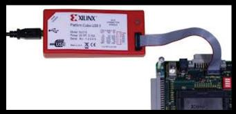
JTAG connection can be used for debugging! Logic analyser cores
