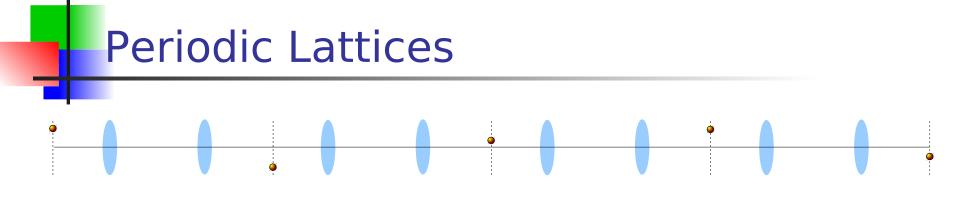
Following n identical cells or turns in a ring with one-turn matrix M
