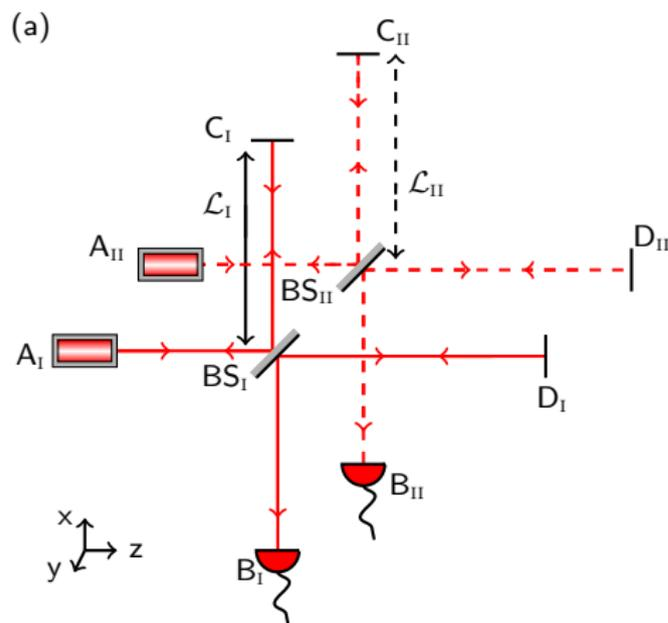
Schematic diagram of the Holometer and QUEST setups.
