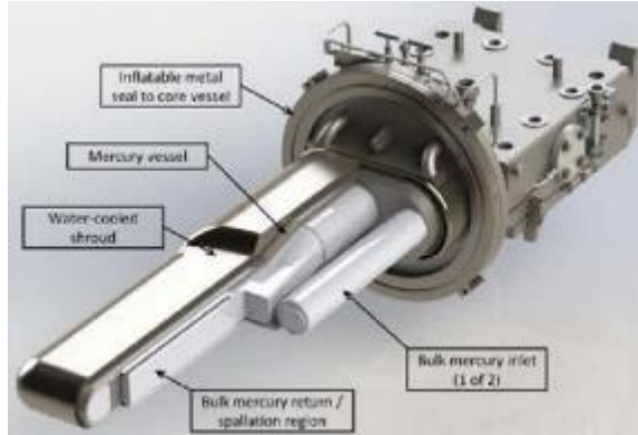
SNS (Oak Ridge) 1 MW liquid mercury target
