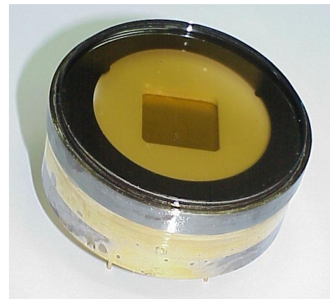
GEM with semi-transparent Photocathode (K-Cs-Sb)
