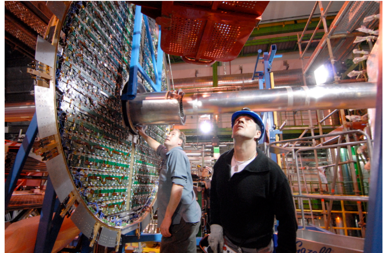
Preshower Dees positioned around beam pipe
