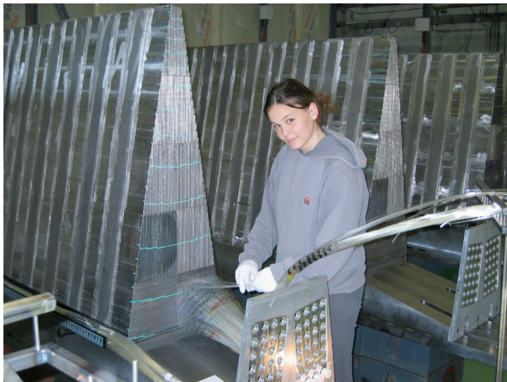
Inserting HF quartz fibres
